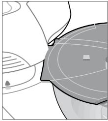
4 Turn the swivel head D clockwise and press to lock securely. Insert the glass bowl pusher N into the filler spout on the glass bowl lid G.
